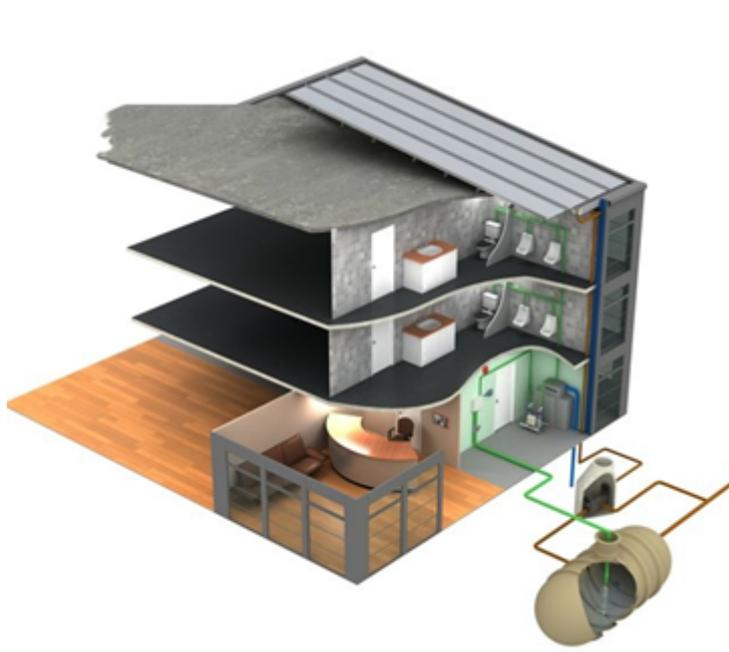
Figure 17. Typical commercial rainwater harvesting system
