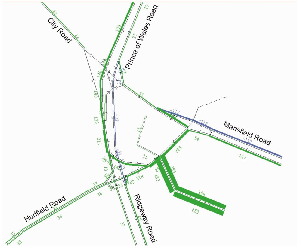
**Figure 8.3 Change in Traffic Flows for Restricted Rerouting (Do Minimum versus Base)**
