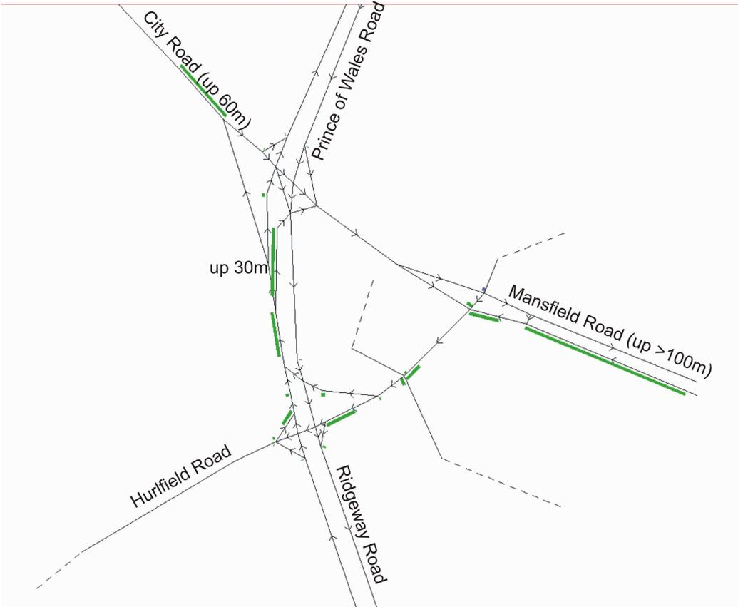
**Figure 8.4 Change in Queue Lengths for Restricted Rerouting (Do Minimum versus Base)**
