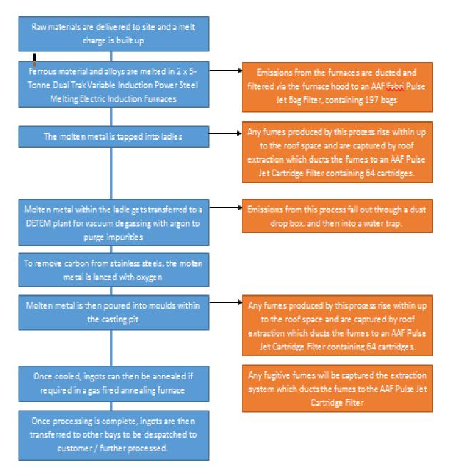
The AAF Pulse Jet Cartridge Filter and the AAF Fabri Pulse Jet Bag Filter are ducted to a single stack. This stack has been fitted with a probe connected to a PCME Dust Alert 25 monitoring system which will continuously monitor the particulate emissions that pass through the stack. This has an alarm feature which is set to sound when it measures a level of  $15 \text{mg/m}^2$  or above.
