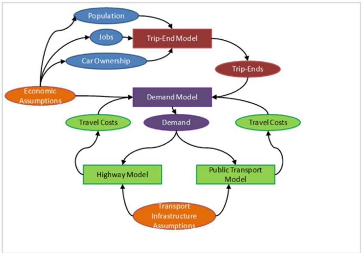
Figure 1. SCRTM1 Model Structure
