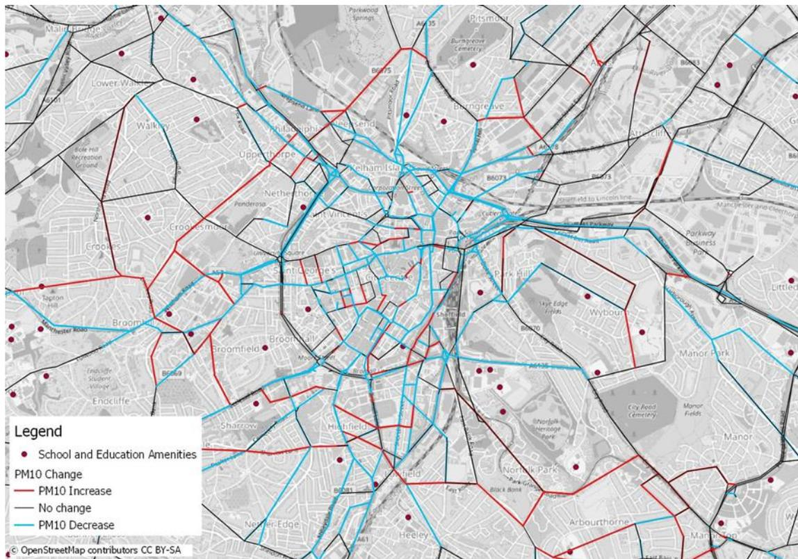
Figure 25. Impact of CAZ on PM<sub>10</sub> emissions around and within CAZ boundary
