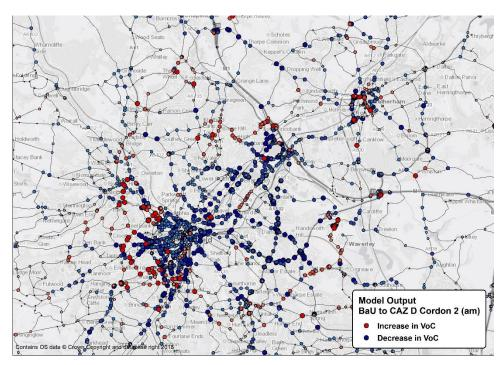
Figure 32 - 2021 Cordon 2 CAZ D – AM Peak Volume / Capacity Changes
