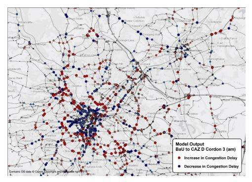
Figure 47 - 2021 Cordon 3 CAZ D – AM Peak Volume / Capacity Changes
