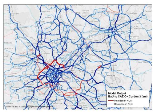
Figure 62 - 2021 Cordon 3 CAZ C+ – AM Peak NO<sub>X</sub> Emissions Changes
