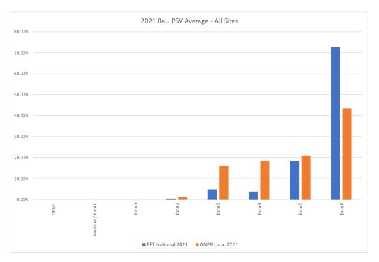
Figure 13 - Sheffield and Rotherham 2021 Passenger Service Vehicle (PSV) Fleet Split
