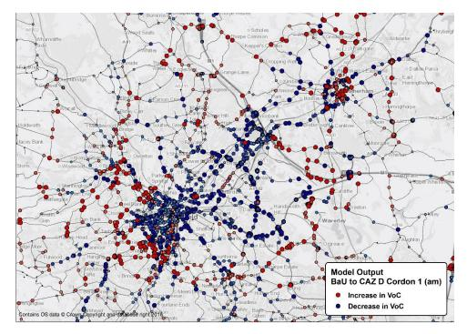
Figure 29 - 2021 Cordon 1 CAZ D – AM Peak Volume / Capacity Changes
