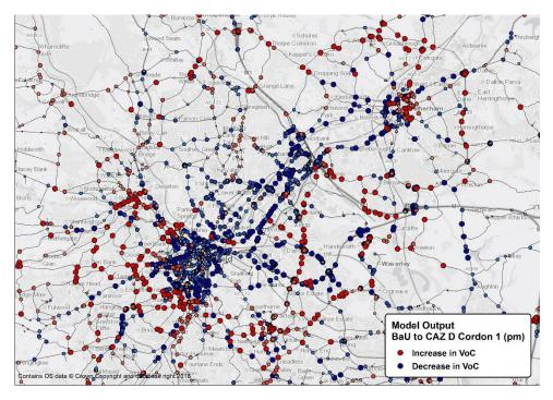
Figure 30 - 2021 Cordon 1 CAZ D – PM Peak Volume / Capacity Changes
