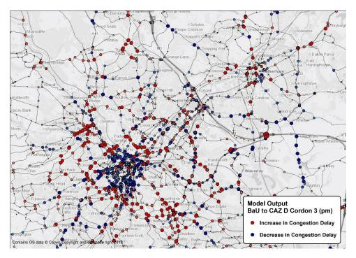
Figure 48 - 2021 Cordon 3 CAZ D – PM Peak Volume / Capacity Changes
