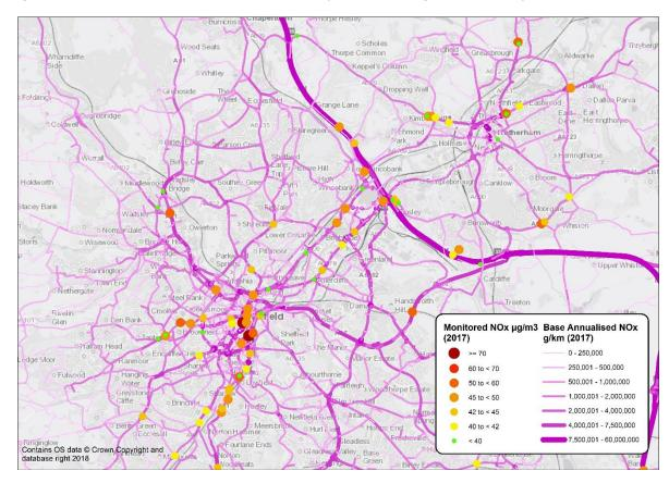
Figure 4. Emissions in the 2017 Base Year model output AQ monitoring sites across study area.
