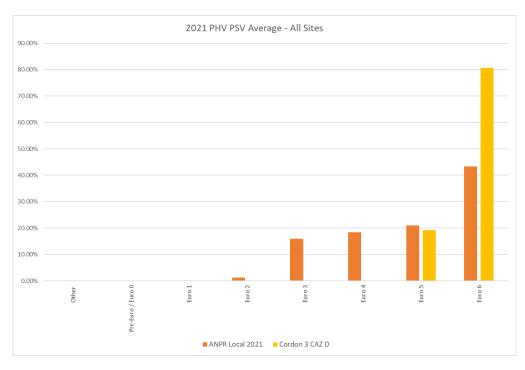
Figure 65 – Changes to 2021 Bus Fleet as part of scheme (Sheffield and Rotherham areas combined)
