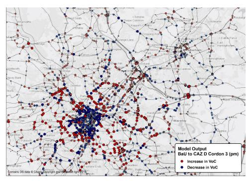
Figure 36 - 2021 Cordon 3 CAZ D – PM Peak Volume / Capacity Changes
