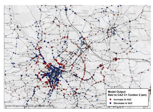
Figure 38 - 2021 Cordon 3 CAZ C+ – AM Peak Volume / Capacity Changes
