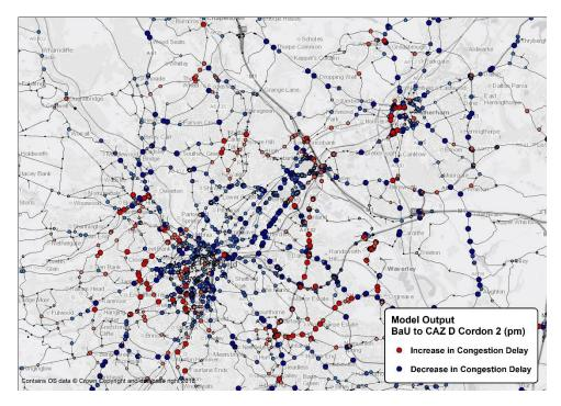
Figure 45 - 2021 Cordon 2 CAZ D – PM Peak Volume / Capacity Changes
