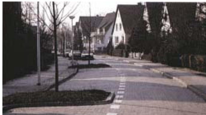
14. Incorporating parking into long streets, e.g. Buchanan Road, with bays between avenue trees (Buxtehude, Germany).
