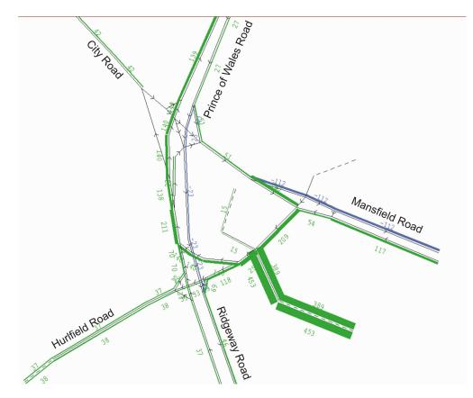
Figure 8.3 Change in Traffic Flows for Restricted Rerouting (Do Minimum versus Base)
