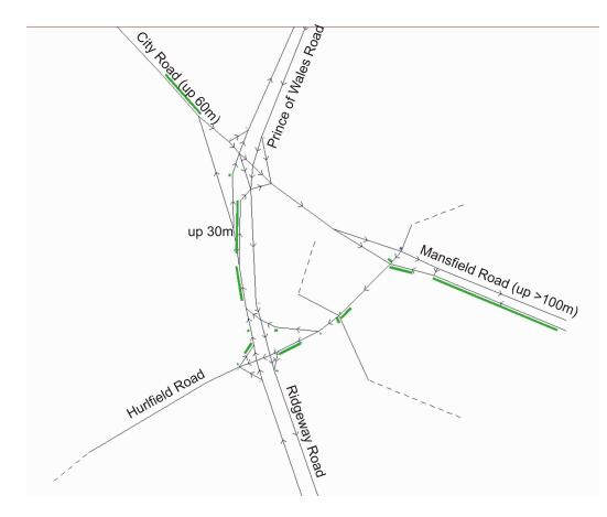
Figure 8.4 Change in Queue Lengths for Restricted Rerouting (Do Minimum versus Base)
