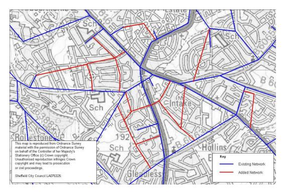
Figure A1 Existing Network with Minor Roads Added for Study
