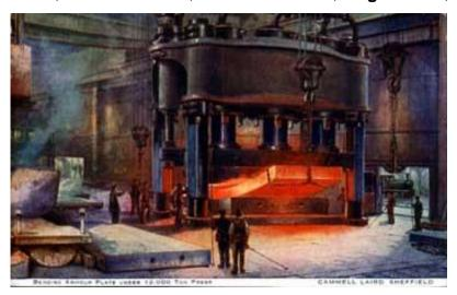
12,000 Tons Armour Plate Bending Press, Cammell Laird & Co. Ltd, Cyclops Steel and Iron Works (Picture Sheffield: s10828)
