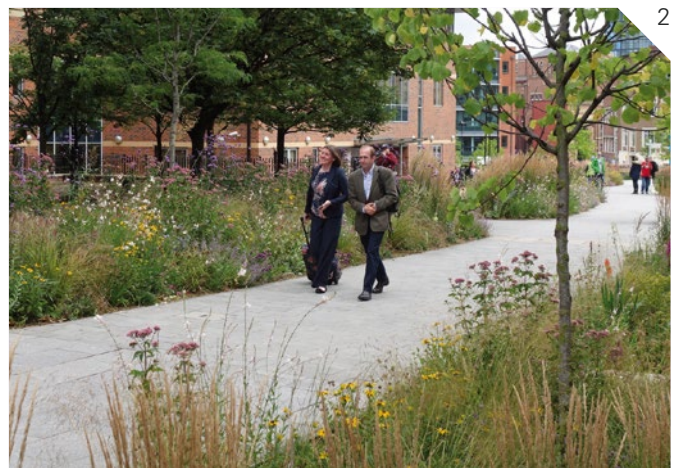
An example of swales managing rainwater and improving biodiversity, whilst creating an attractive walking environment- West Bar, Sheffield
