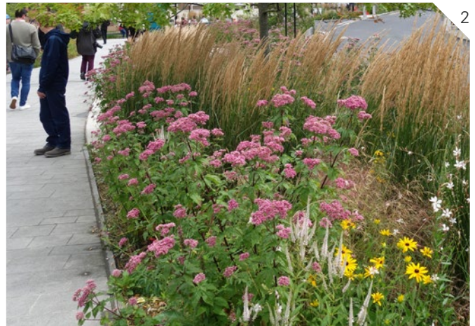
Grey to Green, Sheffield- Example of an attractive green street with SuDS running along the edge of walkways and roads
