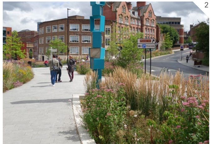
An example of a pedestrian route with SuDS features running along the footpath, with seasonal and verdant planting. Sculptures are incorporated to animate the street. Grey to Green, West Bar, Sheffield
